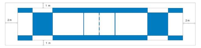
The light intensity around the piste (1 meter along the piste and 2 meters at both ends) must be the same as on the field of play.
