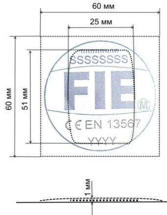
Before sewing of the label, RF tag is fixed in the center on the adhesive layer located on the other side of the label.
