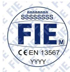
Label represents a bit of fabric with adhesive sub layer, 60x60 mm or 60x35 mm. There is FIE logo on the face side. Label is glued on a paper roll with a wax layer which removes easily.
